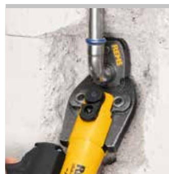
REMS pressing ring 45° (PR-2B) Patent EP 2 774 725
